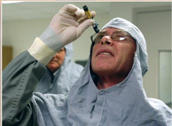
During a training session at HAMMER, a student checks a dosimeter, or gamma pencil. These "pencils" are checked before, during, and after every entry into a radiological area to make sure workers don't exceed limits specified in radiation work permits.
