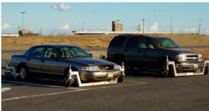
Hanford Patrol now has two vehicles equipped with the SkidCar System to enhance driving skills.
