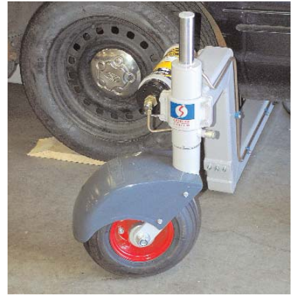
The front outrigger (left) and rear outrigger (right) are strong enough to hold the car completely suspended in the air.
