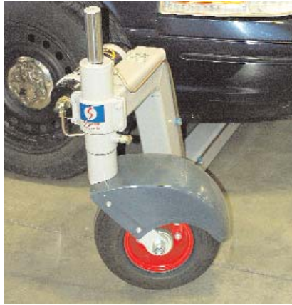
The front outrigger (left) and rear outrigger (right) are strong enough to hold the car completely suspended in the air.
