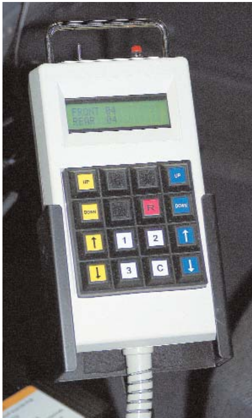
H.A.L., the electronic control box inside the vehicle, allows a Skid Car instructor to individually raise or lower the front or rear outriggers.
